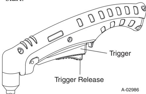
5. Bring the torch within transfer distance to the work. The main arc will transfer to the work, and the pilot arc will shut off.
