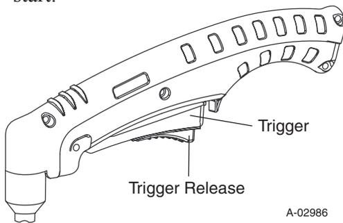
6. Bring the torch within transfer distance to the work. The main arc will transfer to the work, and the pilot arc will shut off.
