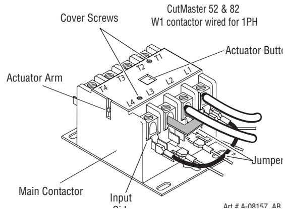
2. Retest continuity between terminals while engaging the contacts manually. This can be done by pushing down on the recessed actuator button on the top of W1 or pushing down on the actuator arm on the side of W1.
