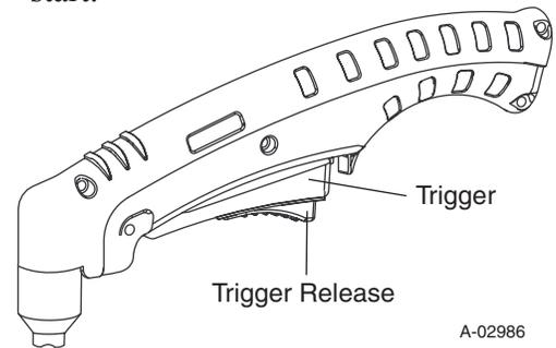
7. Bring the torch within transfer distance to the work. The main arc will transfer to the work, and the pilot arc will shut off.
