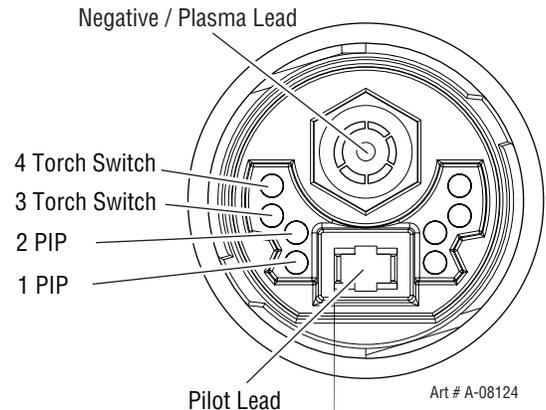
If a short is found, the problem is in the torch and leads assembly. Remove the torch head from the leads and check the leads and head to determine which is defective.
