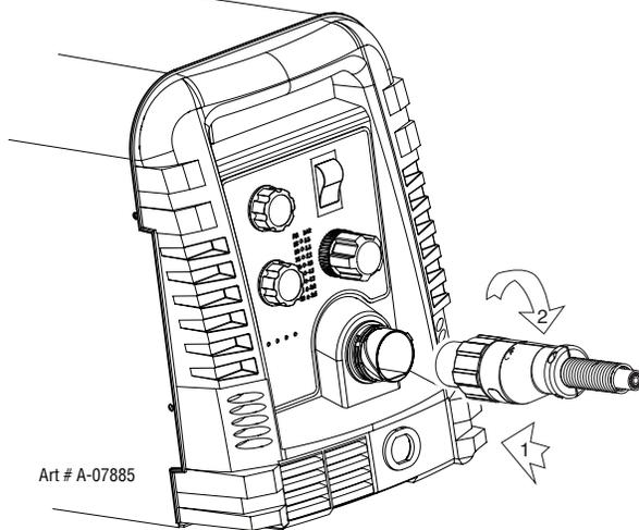
Connecting the Torch to the Power Supply
