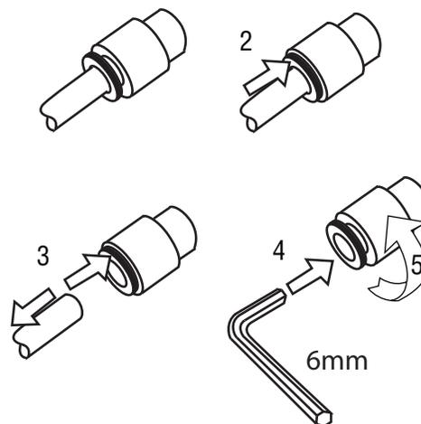
5. Remove the fitting from the filter element assembly by inserting a 6 mm hex wrench into the internal hex fitting and turning it counter clock-wise (left). Numbers 4 and 5 in the previous illustration.
