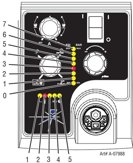
When the "Fault" indicator is on or blinking it will be accompanied by one of the pressure indicator lights depending on what the Fault is. Only one of these faults will be displayed at one time. If more than one fault exists, when the first fault is corrected and cleared, the next fault will then be displayed. It is possible to have a fault indicated in the function indicators and another fault indicated in the pressure indicators. The following table shows each of the Faults possible.
