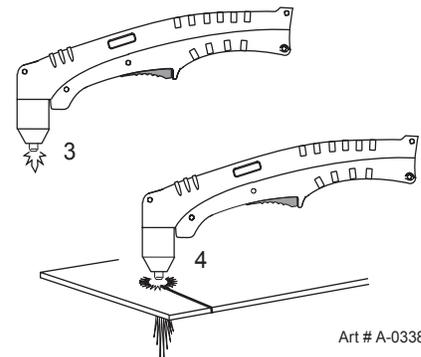
8. Cut as usual. Simply release the trigger assembly to stop cutting.
