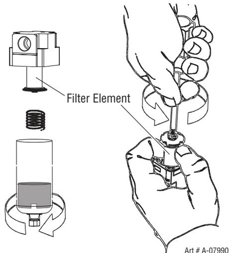
8. Install the new or cleaned assembly by reversing these procedures.
