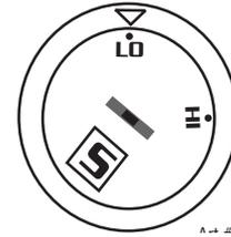
**PART IN PLACE:** Indicates that the shield cup is not properly installed or tightened.
