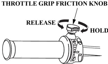
The throttle grip friction knob adjusts resistance to throttle grip rotation.
