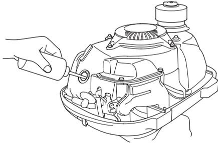
5. Pour a teaspoon of engine oil into the spark plug hole, and then pull the starter grip several times to lubricate the inside of the cylinder.
