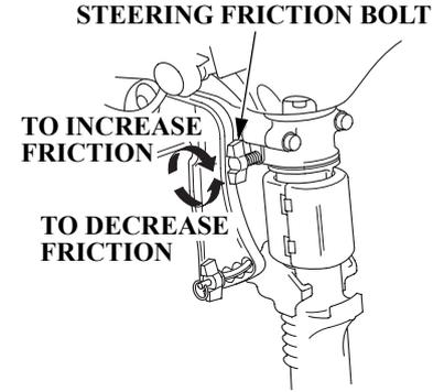
The steering friction bolt adjusts steering resistance.
