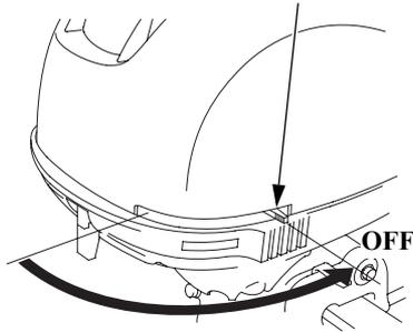
3. Move the fuel valve lever to the OFF position.
