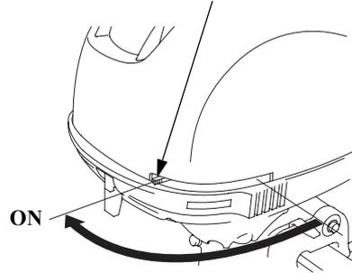
3. Move the fuel valve lever to the ON position.
