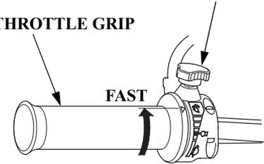
Use the throttle grip friction knob to help hold a constant throttle setting while cruising.
