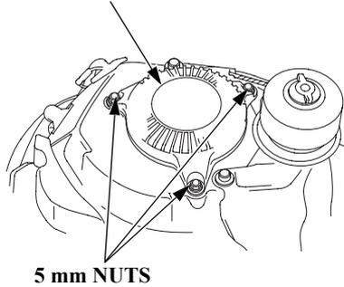
2. Remove the three 5 mm nuts with an 8 mm wrench and remove the recoil starter.
