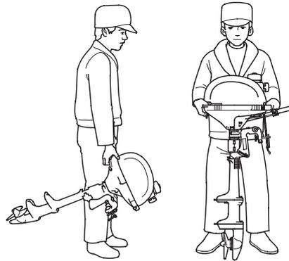
To carry, hold the outboard motor by the carrying handle, as shown.
