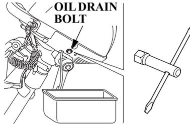
4. Remove the oil drain bolt and O-ring to drain the oil.
