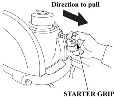
6. Pull the starter grip lightly until you feel resistance, then pull briskly in the direction of the arrow as shown above.
