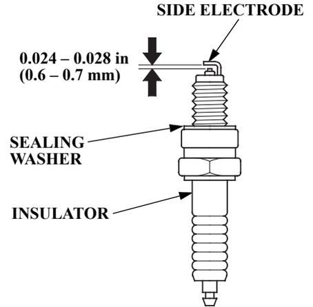
5. Measure the spark plug electrode gap with a wire-type feeler gauge. Correct the gap, if necessary, by carefully bending the side electrode.
