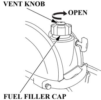
The fuel filler cap is provided with a vent knob to seal the fuel tank. Open the vent by turning the vent knob to the ON position before starting the engine (p. 25).
