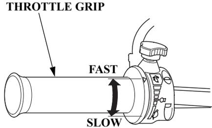
The throttle grip controls engine speed.
