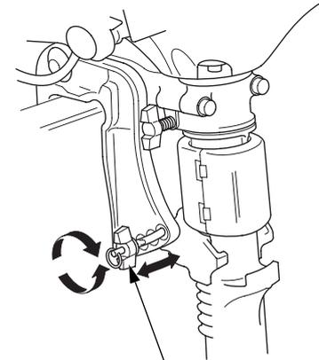
ADJUSTING BOLT AND WING NUT
