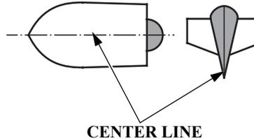
Install the outboard motor on the center of the boat transom.
