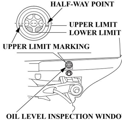
Use the oil level inspection window to check the engine oil level with the engine stopped and the outboard motor in the upright position.
