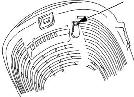
4. After draining is completed, tighten the carburetor drain screw and turn the fuel valve lever to the OFF position.
