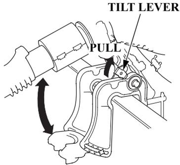
5. To return the outboard motor to the normal running position, hold the outboard motor by the front carrying handle on the engine case and pull the tilt level toward you, and then lower the outboard motor slowly.
