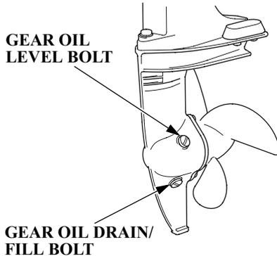
1. Place a suitable container below the oil drain hole to catch the used oil, then remove the oil level bolt, oil drain/fill bolt and washers.
