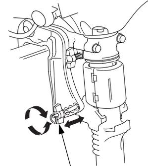
The transom angle adjusting bolt is used to adjust the angle of the outboard motor in the normal operating position (see page 34).
