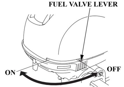
The fuel valve opens and closes the passage between the fuel tank and the carburetor.
