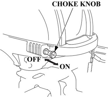
The choke knob opens and closes the choke valve in the carburetor.
