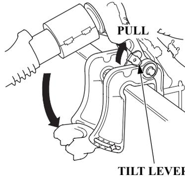
To return the outboard motor to the normal running position, hold the outboard motor and pull the tilt lever, then slowly lower the outboard motor.
