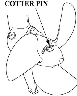
Install the propeller in the reverse order of removal. Be sure to replace the cotter pin with a new one.
