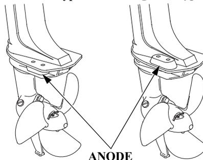
The anode is made of a sacrificial material that helps to protect the outboard motor from corrosion.
