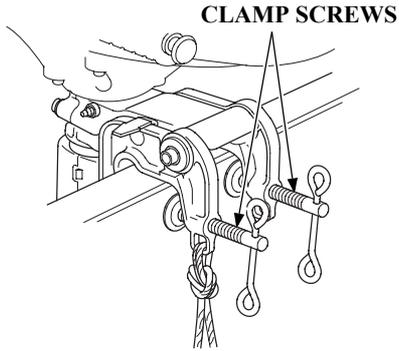
Use the clamp screws to secure the outboard motor to the transom.
