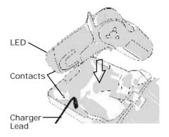
The LED light on the handle of the POWERmini driver will turn red while the battery is charging and turn off once the battery is fully charged.
