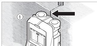
When an object is indicated directly below the center line **k** in display **16**, as in the example, mark it roughly with the top marking guide **1**. This mark will only be precise when the object is positioned exactly vertical in the wall, as the sensor range is
