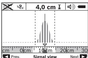
The object depth and the material types (as far as possible) are displayed. The maximum measuring depth is 6".
