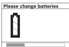
When the “Please change batteries” warning indication is shown on the display **16**, the settings are saved and the detection tool switches off automatically. Measurements are no longer possible. Change the batteries.
