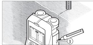
For exact marking of the object on the wall, move the detection tool left or right until the found object is positioned below one of the outer edges. When the found object is indicated directly below the dashed righthand line **g** in display **16**, mark it with the right marking aid **3**.
