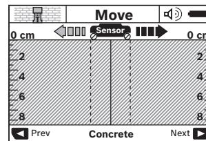
Position the detection tool against the wall and move it over the wall in the direction of travel (see "Operation Instructions", page 13). Measured results are indicated on display **16** after a minimum measuring distance of 4" (10 cm). To ensure correct measurement results, move the detection tool slowly and completely over the assumed object in the wall.
