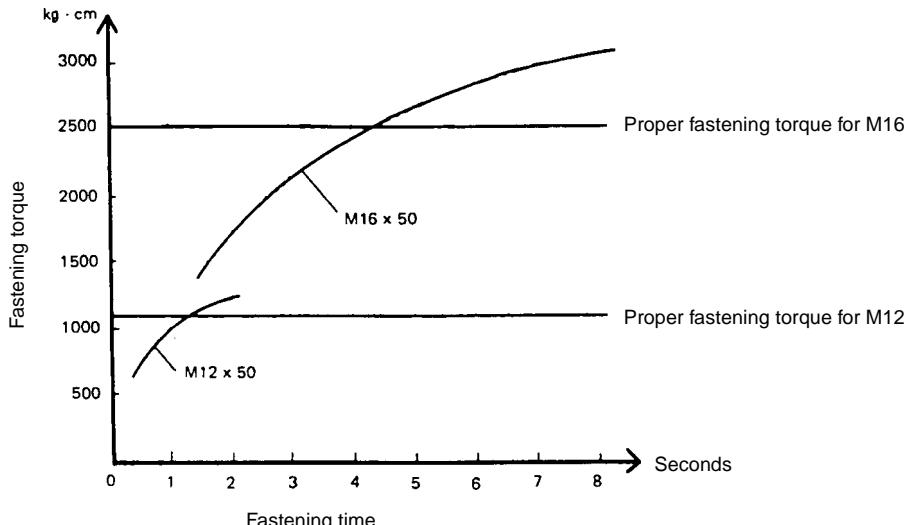
Hold the tool firmly and place the socket over the bolt or nut. Turn the tool on and fasten for the proper fastening time.
